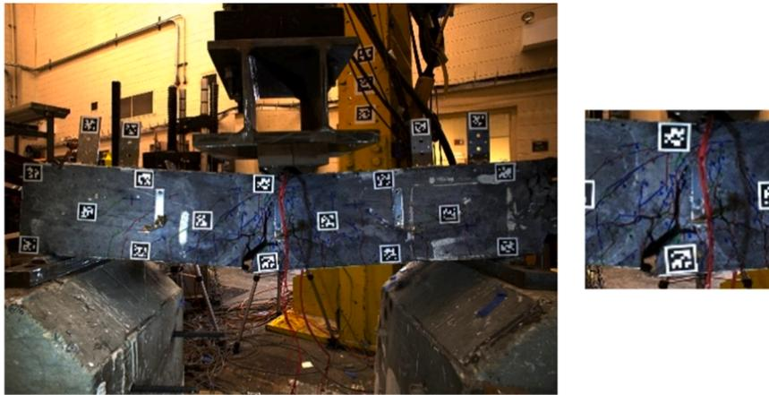
Fig. 11. Photo of G4N physical specimen at time 3500 s. Partial detachment of UHPC with attached AprilTag (tag-19) at the bottom of the section was observed due to severe cracking.
